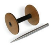
The Majacraft stylus is a polished aluminium quill or spindle that screws straight on to the flyer shaft. A small bobbin is part of the set and is placed on the shaft first with the stylus snug against it. Make sure the stylus is done up quite tightly so that it doesn't come undone when working. You can treadle it on and off just as with your flyer. The stylus attachment will fit all Majacraft spinning wheels.
